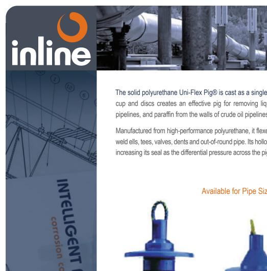
The solid polyurethane Uni-Flex Pig® is cast as a single piece construction. The flexible combination of cup and discs creates an effective pig for removing liquids from wet gas systems, water from product pipelines, and paraffin from the walls of crude oil pipelines.
