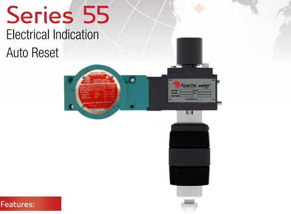
Base Model 55-0000 are an electrical indicator with automatic reset. It includes a thread mounting nipple, standard lower housing with fluorocarbon O-Rings, hemispherical plunger and weather sealed & explosion proof limit switch. The switch employed on this model is NEMA rated, UL listed and CSA certified to suit most applications.
