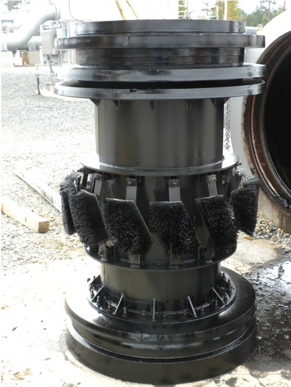
Figure 7: Standard Hard Bodied Cleaning Pig as received at Vernon
