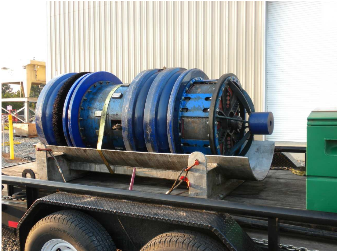
Figure 8: SCP 42 inch tool cleaned and ready for launch in the next pipeline section at Vernon
