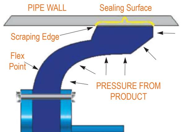
The design of the DC Cup<sup>®</sup> surface bearing area and the flex area provides maximum wear resistance.
