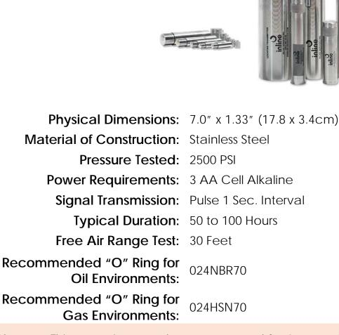
Note: This transmitter can be programmed for 2 second pulse intervals, thereby doubling the duration time of doubling the power (increased range) for the same duration. Also, continuous mode is possible at ½ duration, if programmed for this mode.
