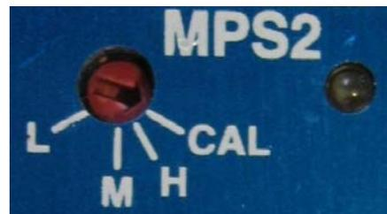
Once the sensor has finished its calibration, the LED will begin double blinking every 2 seconds. This indicates successful calibration.
