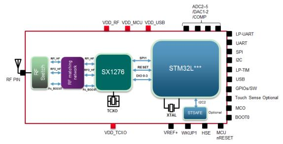
None of the port pins made available on the Murata CMWX1ZZABZ-078 module are connected on the 4003 LoRa PCB. The user can configure these pins as desired possibly for debugging purposes as pads connected to these pins are made available on the 4003 LoRa PCB.
